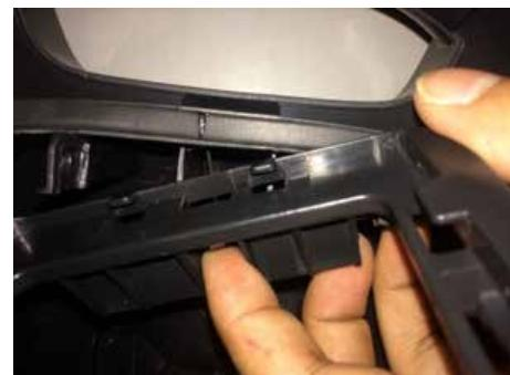
03. Open the front cover and tap the bottom area to remove the front cover.
