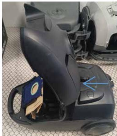
06. Push up to remove air inlet filter.
