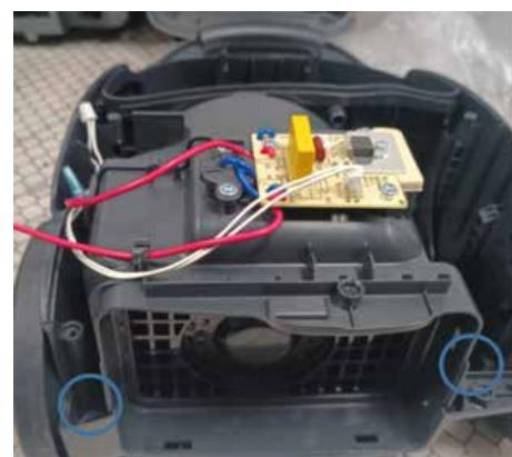
09. Remove the connector of the potentiometer on the back cover and the connector of the switch.
