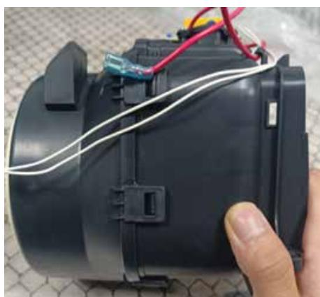
16. Remove two screws,take down pressing plate then remove switch.
