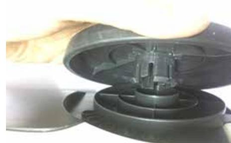
21. Reverse swing latch to remove the front cover latch.
