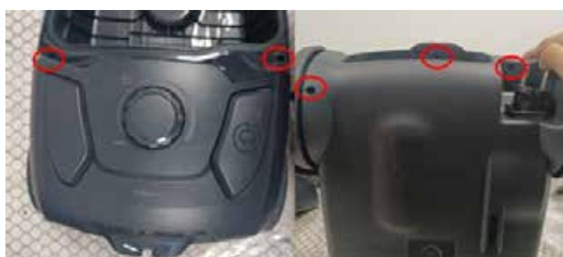
11. Remove 2 screws, pull motor cover upward and take out motor assembly.
